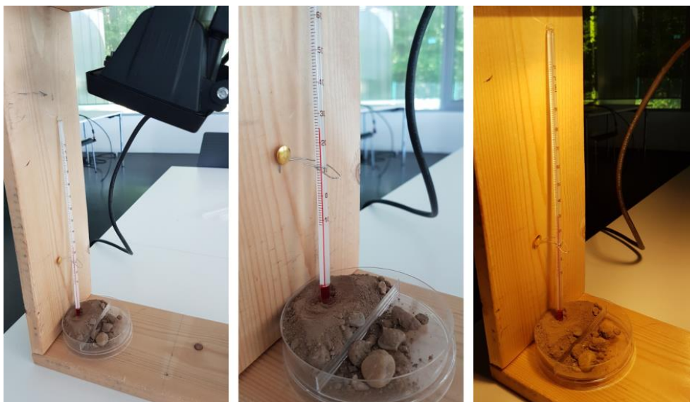
Figure 9: The set-up of the second experiment is the same as for the one with water, but this time the petri dish is filled with dirt, sand, or soil (own work).
