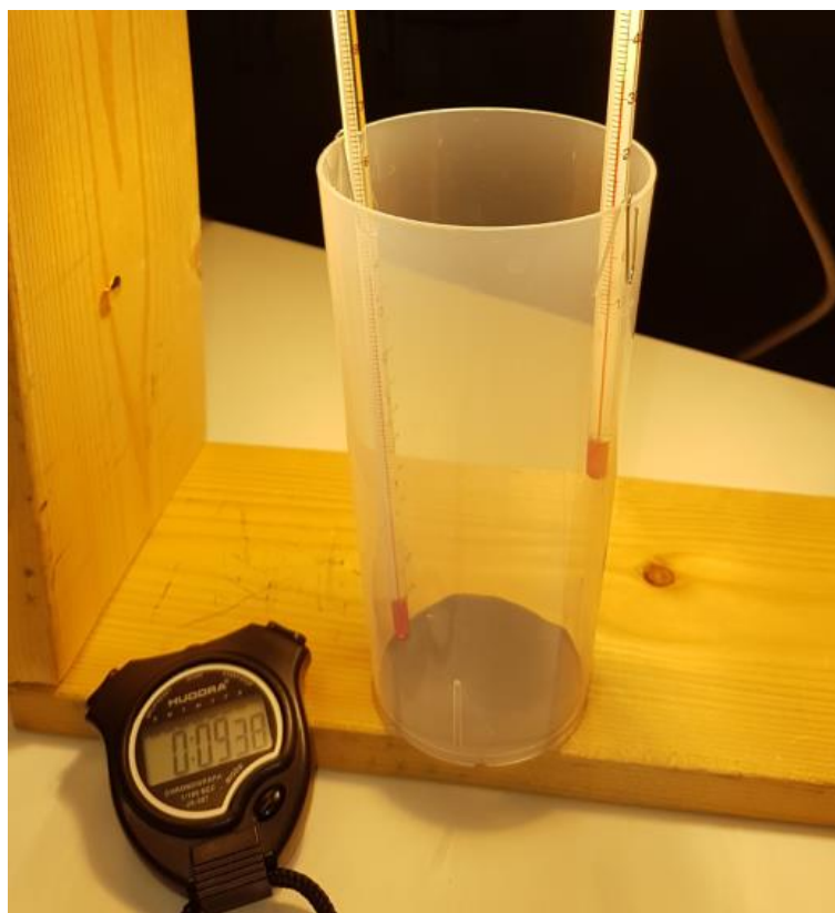
Figure 10: While illuminated, the temperatures are read off the thermometers every minute (own work).
